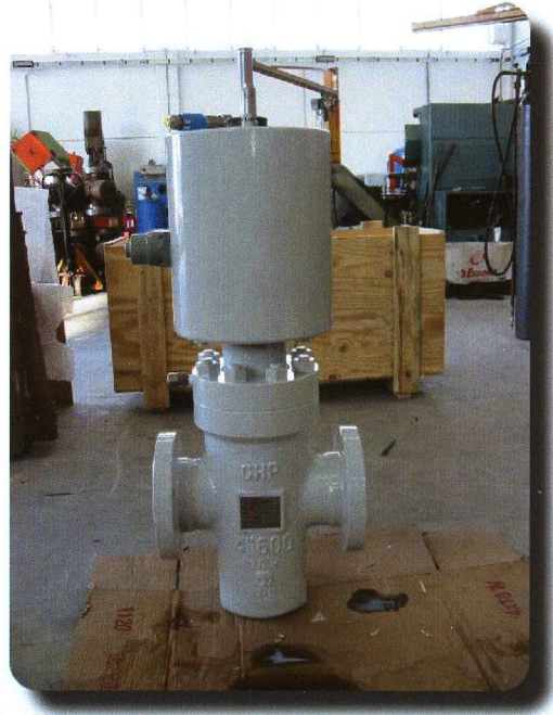
GATE VALVE 4" 600 with Pneumatic Actuator
